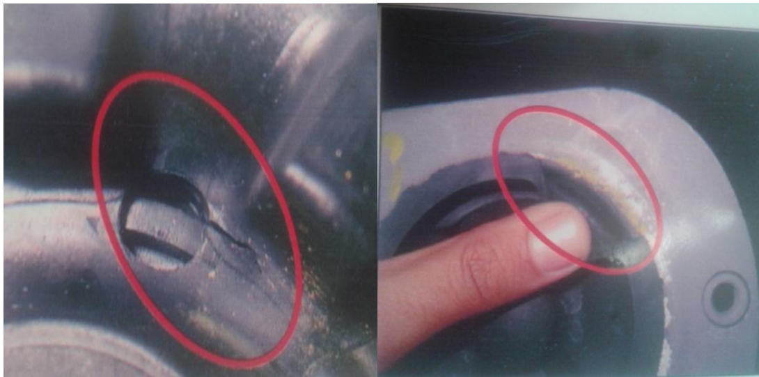
Fig. 5: Rubber crack and Loose bond defects
